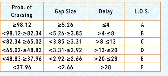
L.O.S. standards based on Delay & Gap Size.
